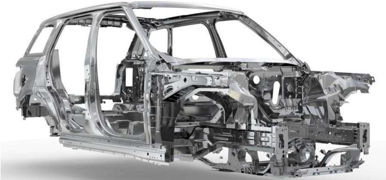
*Figure 2 An all-aluminium automotive body-in-white structure.*
