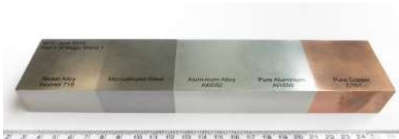
Figure 2 - Nickel alloy welded to steel, welded to aluminium alloys, welded to copper by LFW.
