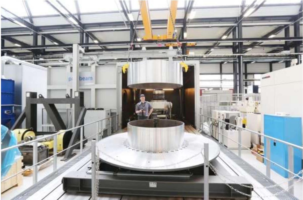
*Figure 2 – Large Scale Electron Beam Welding*
