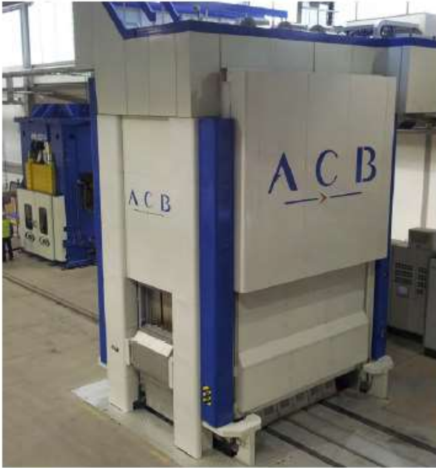
Figure2: ACB 1200T superplastic forming/600T Hot creep forming press at AFRC
