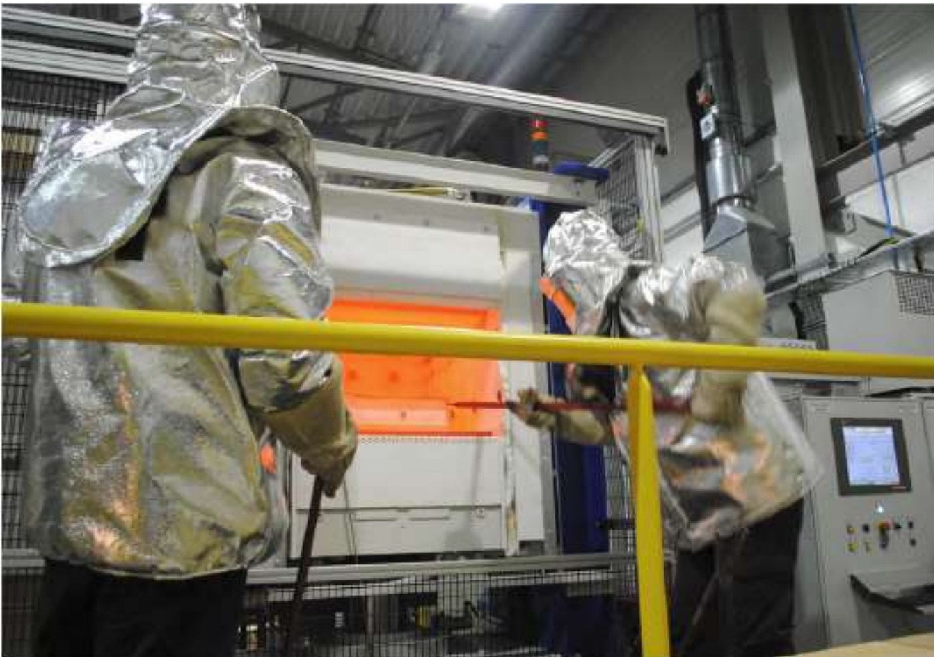
Figure1: ACB Loire 200T superplastic and diffusion bonding press at AFRC
