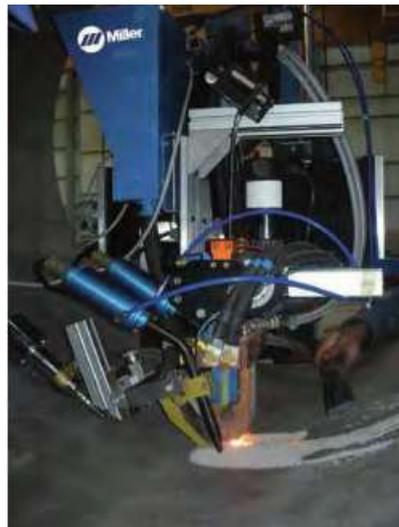
*Figure 4 Miller Electro-Slag Strip Cladding of a vessel internal surface*
