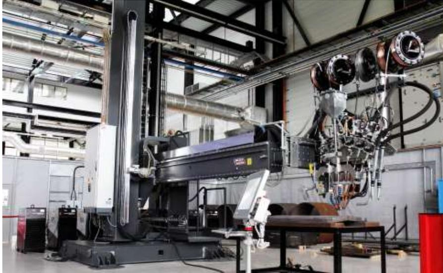
*Figure 3 PEMA Multi-wire SAW system set-up*
