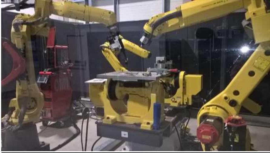
*Figure 1 Robotic GTAW and CMT welding cell*
