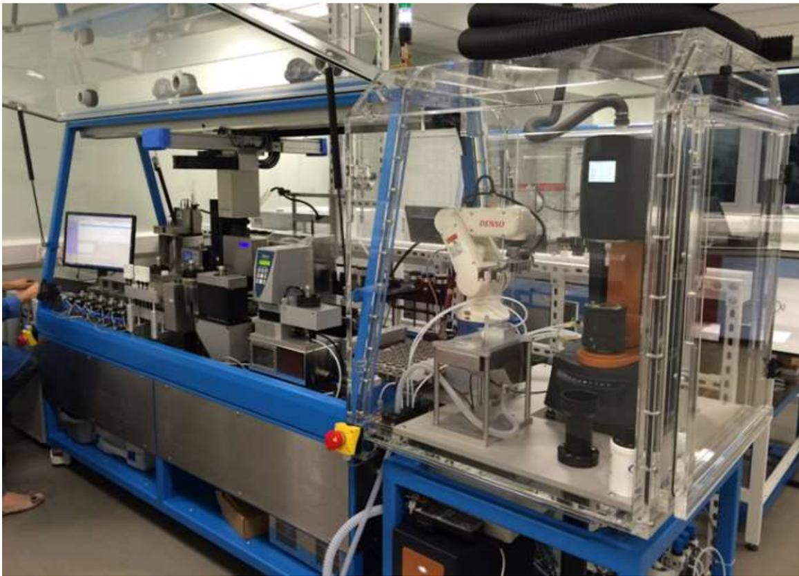
*Figure 1. Robotic formulation platform enabling automated dispense and mixing of solid and liquid materials enabling screening of formulation spaces.*
