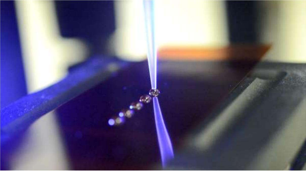
*Figure 3 – Drop shape analysis to determine surface energy of substrates for adhesion*
