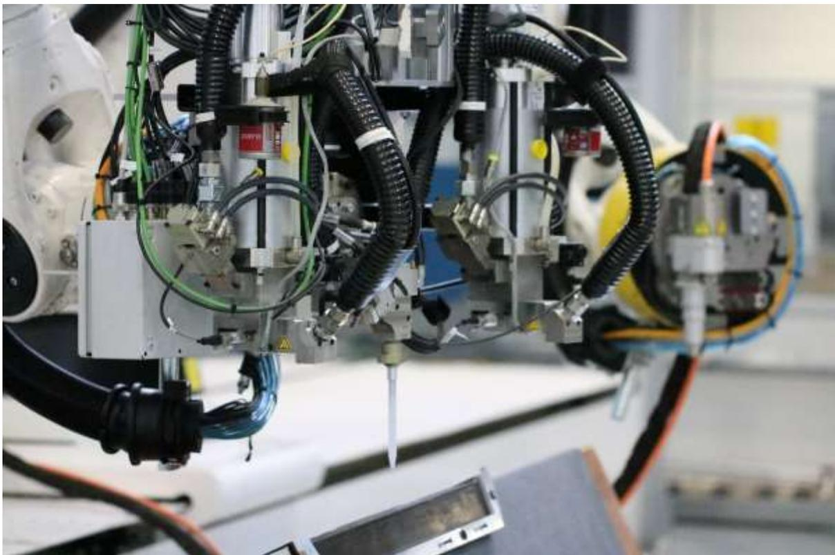
*Figure 2 – Automated application of adhesive for repeatable high rate processing*
