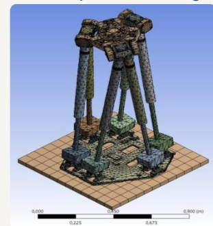
Figure 6: FEM model of the hexapod robotic milling unit assembly
