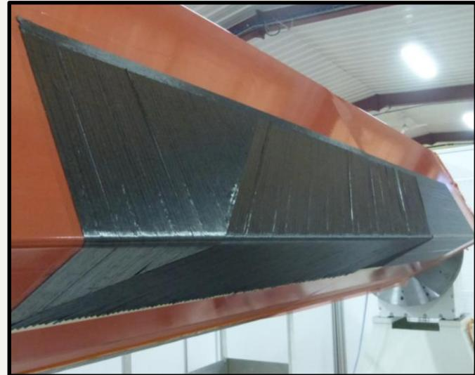
Figure 9: Flat dry fibre preform, including steered tow, laid up with flashlamp
