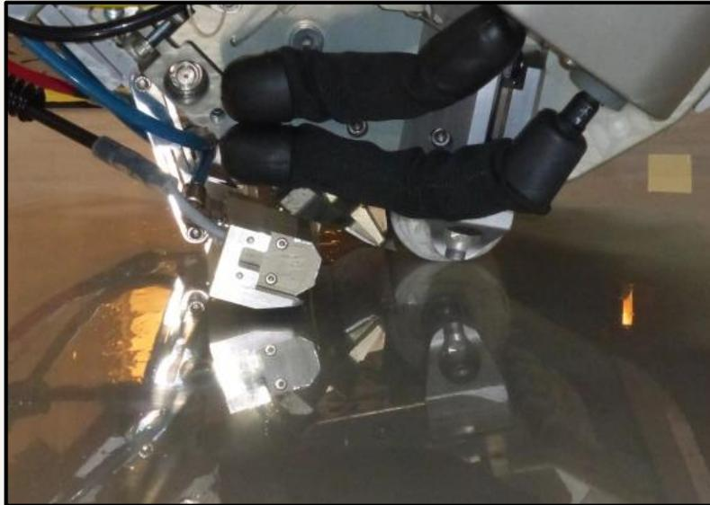
Figure 7: The redesigned Flashlamp mounted to the AFP robotic system
