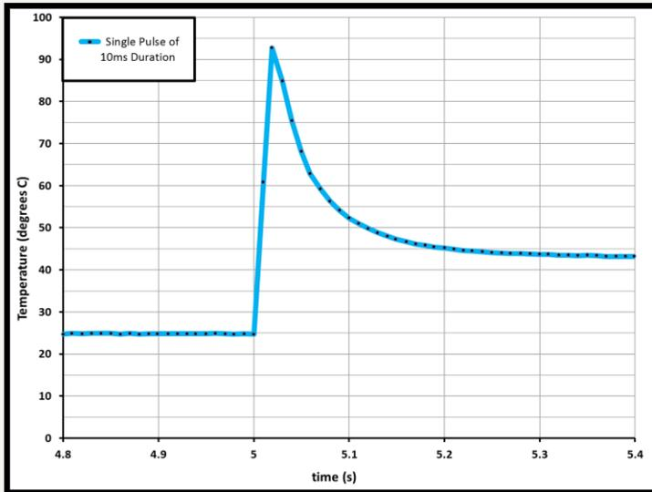
Figure 1: Temperature vs. Time results for a single 10ms Pulse
