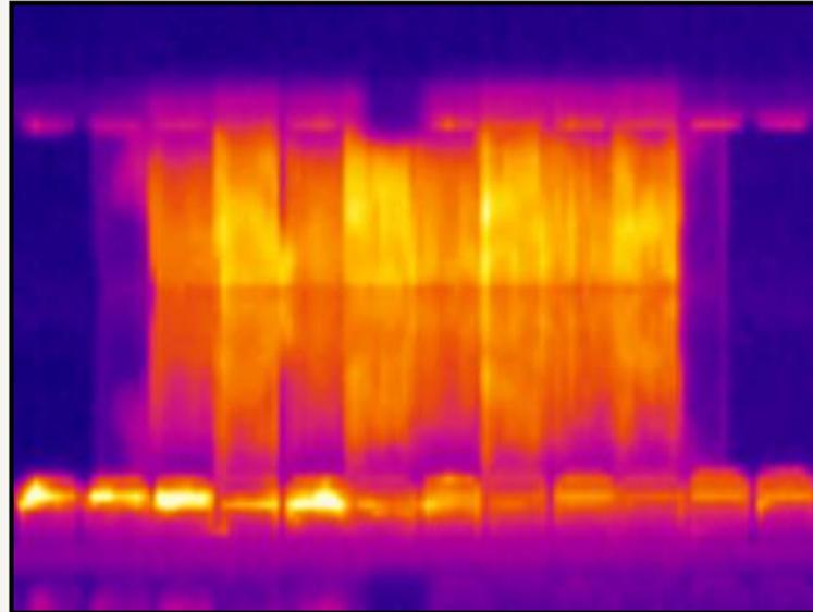
Figure 8: Thermal Image showing the heating of 8 parallel tows
